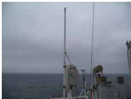
Fig. 4. SSB antenna above bridge and detached antenna shown on deck afterwards
